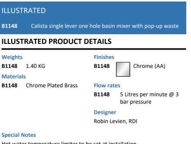
Hot water temperature limiter to be set at installation. Regulated flow rate 5 litres per minute at 1 bar.
